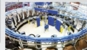
2010 AMR DeLaval launches the first automatic milking rotary. Capacity to milk 90 cows/hour or 540 cows three times/day or 800 cows twice a day.
