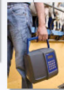
2003 DCC DeLaval coil counter DCC is launched, enabling farmers to measure SCC on the farm in less than one minute.
